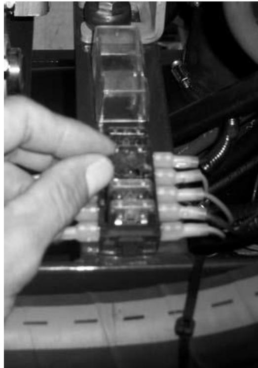
**Fig. B - fuse # 3 removal**
